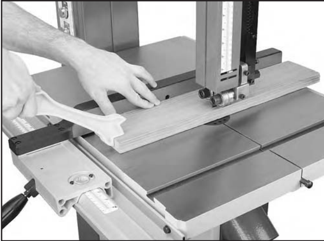
Figure 39. Ripping with a push stick.
