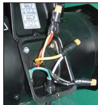
Figure 71. Motor wiring at 220V.
