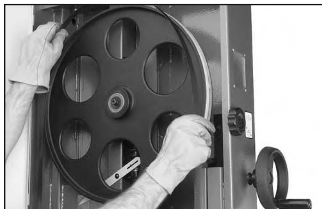
Figure 48. Placing blade on the wheels.
