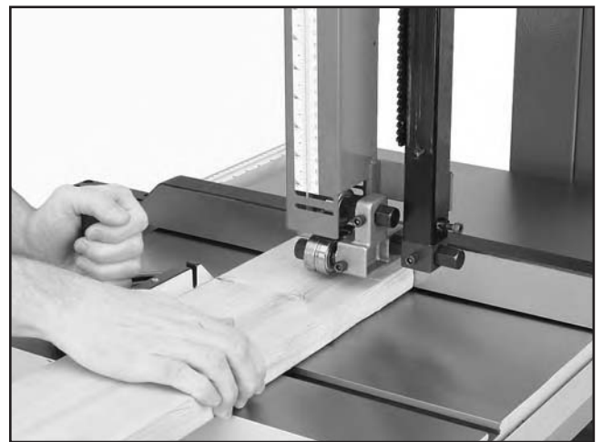
Figure 40. Crosscutting with miter gauge.
