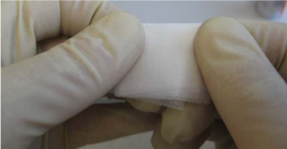
Figure C-4. Fiber End-Face Cleaning
