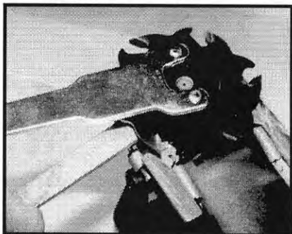
Photo 5.1 Using the pair of wrenches to remove the blade.
