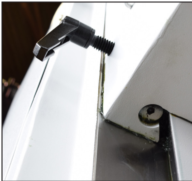
Figure 4-15 Knee gib, underside
