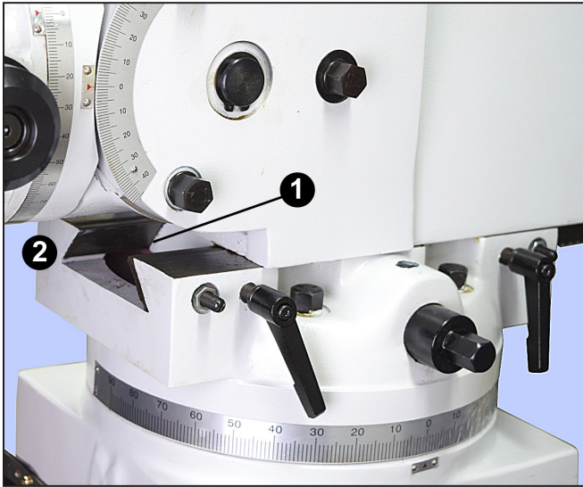
Figure 3-9 Not-to-exceed point When backing the ram, stop when the separation between the forward edges of male and female dovetails, points (1) and (2), is 2-1/2". Go no further. Otherwise, the ram will likely jam and cannot be brought forward unless unweighted by lifting on the eyebolt shown in Figure 3-5.
