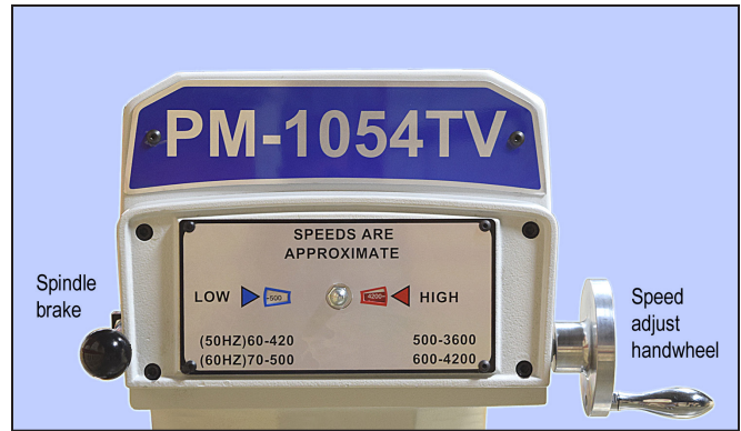
Figure 3-13 TV speed adjustment Turn the handwheel only when the spindle is running
