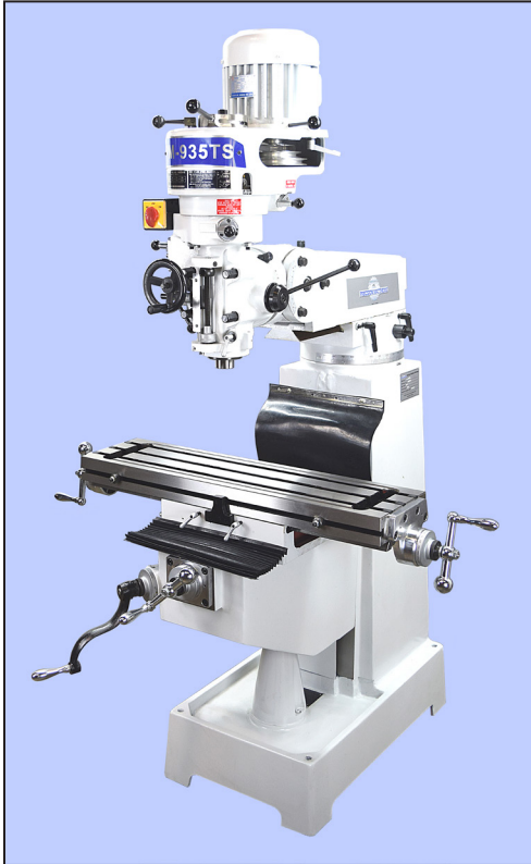
Above: PM-935TS knee mill with 9 x 35 inch table, 8-speed step pulley drive and 3Ø motor (option)
