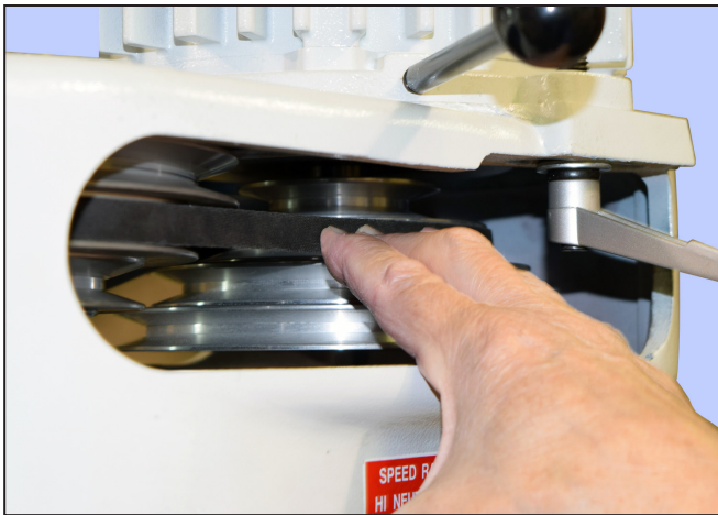
Figure 3-11 Switching from LO to HI range One way to make sure the drive system is properly set before switching on the motor is to push back on the belt with fingertips until you hear the clutch engaging.
