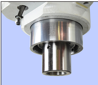
Figure 4-9 Collet locating screw(s)
