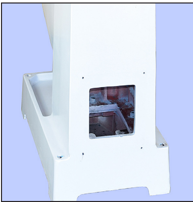
Figure 4-19 Cutting fluid reservoir & pump housing
