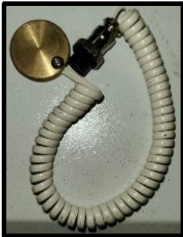
Contact Button of the Tool Touch Off Puck.
