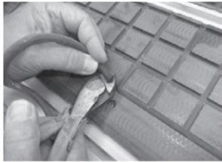
Cutting end of foam rubber gasket
