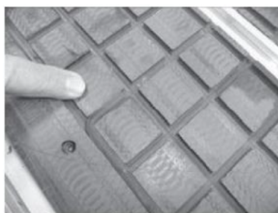
Start point foam rubber gasket turned in
