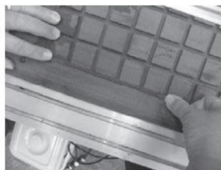
Inserting foam rubber gasket
