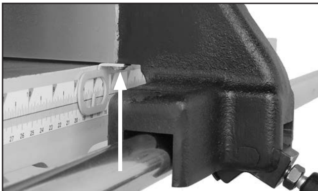
Figure 42. Fence pointer adjustment screw.
