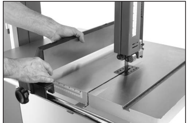
Figure 25. Example of installing fence onto rail.
