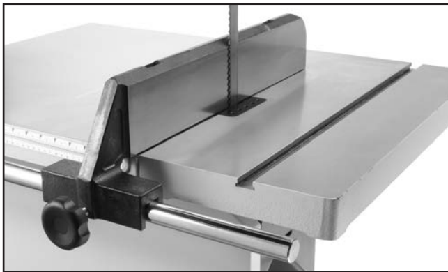
Figure 41. Example of fence flush with blade.
