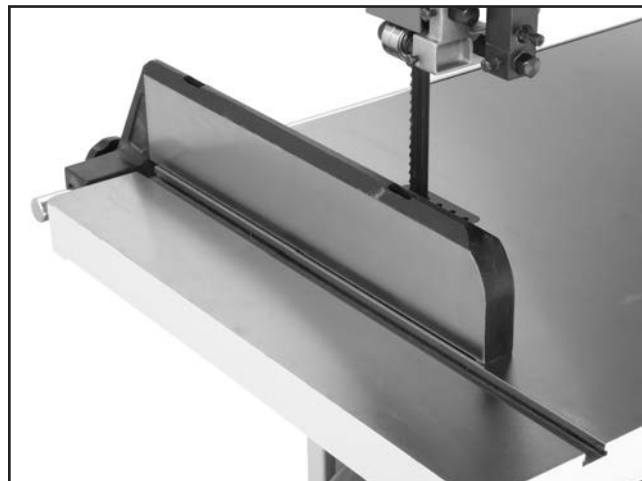
Figure 40. Example of fence square with miter slot.
