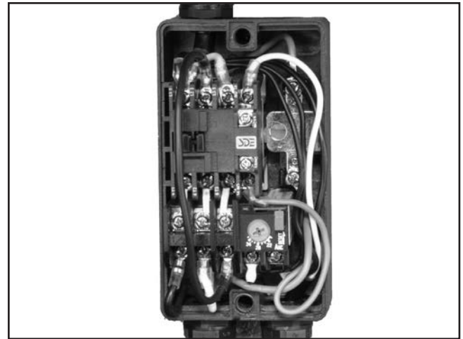
Figure 15. 220V magnetic switch
