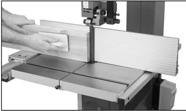
Figure 58. Example of resawing lumber.
