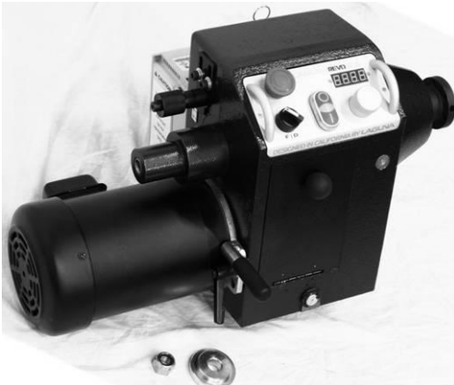
Headstock removed from the bed
