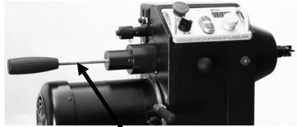
Drive center removal shaft
