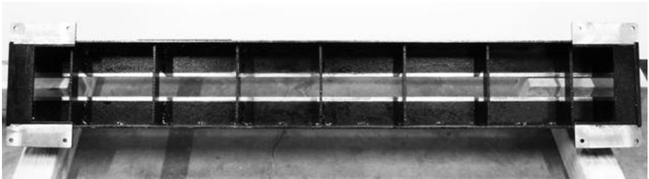
Underside of lathe bed
