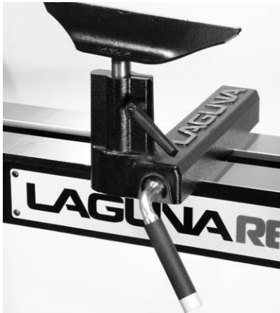
Tool rest assembled to the bed
