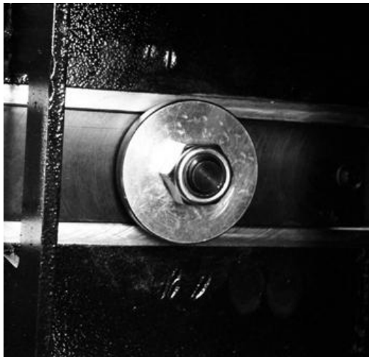
Washer assembled in position
