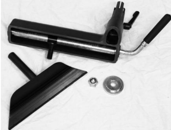
Tool rest unassembled
