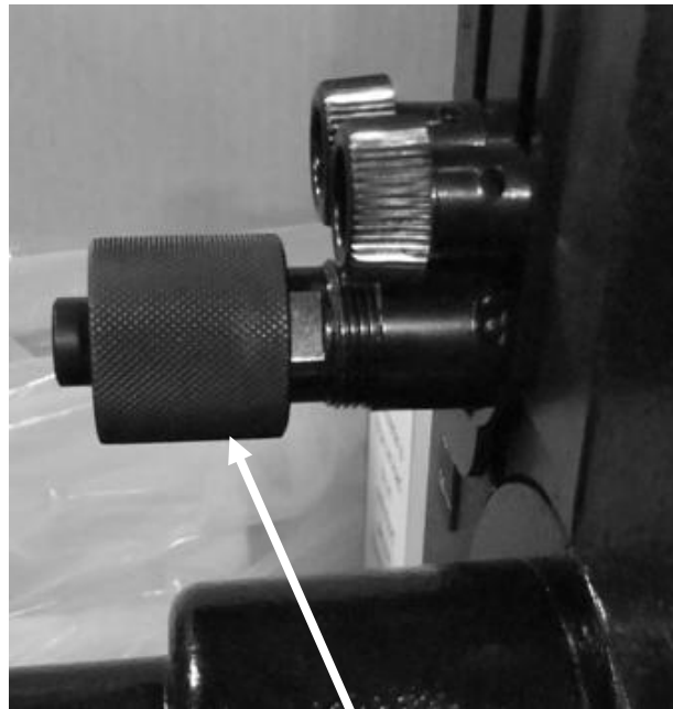
Indexing plunger disengaged
