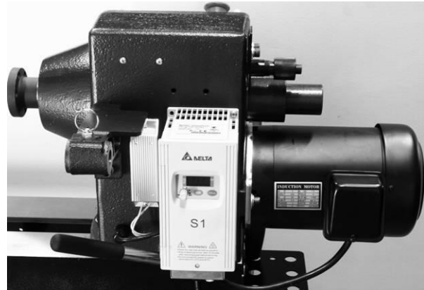
Headstock attached to bed
