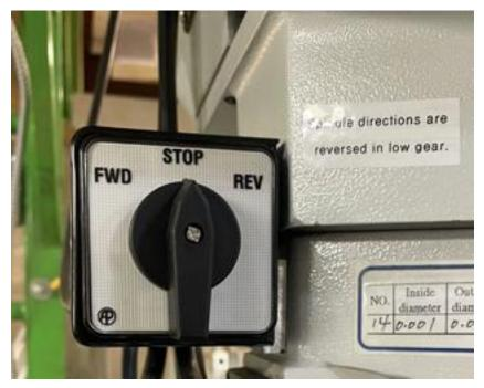
To start the mill, simply turn the power knob to run the spindle forward (FWD) or in reverse (REV).
