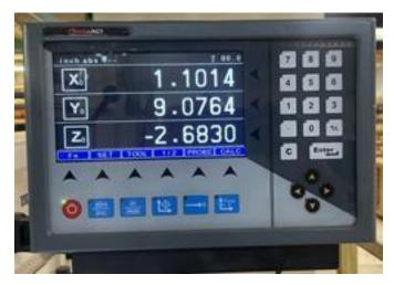
The DRO's basic functions are nearly identical to the Rong Fu's; it just has a three axis readout rather than two. If the DRO doesn't seem to be acknowledging a keypress, try hitting the Clear (C) button and trying again.
