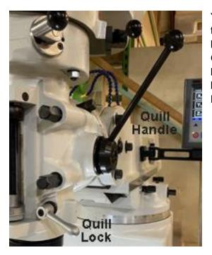
You can raise and lower the quill just like a drill press, with this handle. Like a drill press, and unlike the Rong Fu, it has a spring which will retract it whenever it isn't locked. Generally, you'll use this only for drilling. You will want to keep it locked in a single position for milling operations, because moving it invalidates the Z values shown in the DRO.
