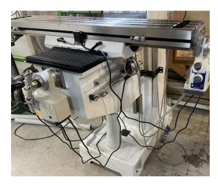
There are many cables and pipes running around the machine's table. These cannot be managed more tightly, as they must be free to move as needed to match the table's large range of motion. Try to be aware of their movements and ensure that they don't catch on or get caught between other parts as the table moves.
