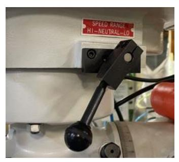
Any lever location between the two detents is neutral, which is useful if you want the spindle to move freely. (On the Rong Fu, you can turn the spindle while it is in gear; you cannot do so here.)
