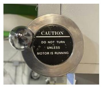
You can adjust the speed setting by turning the wheel on the upper right side of the head.
