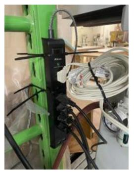
To use the mill, you'll need to power the ancillary features by turning on this power strip, behind the machine to the left. This will provide power to the three auto-feed motors, the DRO (location readout), a spindle light, and a coolant pump which will be installed later.
