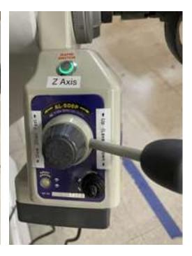
Just like the Rong Fu's feed, these have auto-stops at both ends. However, unlike the Rong Fu, these aren't the hard limit stops for the table travel. You can go a bit further using the manual handles, but this should generally be avoided. Care should thus be taken using manual feed near the table limits.
