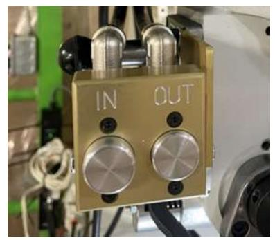
To use it, you do have to make sure the quill is fully up and locked. Insert the collet with the tool in it, aligning the slot on the collet so it travels most of the way in. Then you hold down the IN button until the tool is in place, which will take less than a second. Don't continue to hold the button down beyond that point. To remove the collet, just press the OUT button until the collet is free. This will take slightly longer. The whole system is simple and fast.
