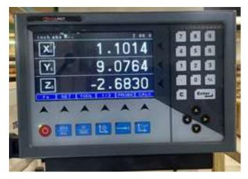
The DRO's basic functions are nearly identical to the Rong Fu's; it just has a three axis readout rather than two. If the DRO doesn't seem to be acknowledging a keypress, try hitting the Clear (C) button and trying again.
