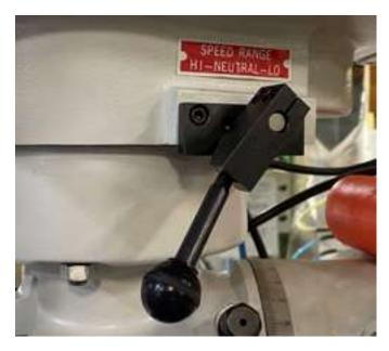
Any lever location between the two detents is neutral, which is useful if want the spindle to move freely. (On the Rong Fu, you can turn the spindle while it is in gear; you cannot do so here.)
