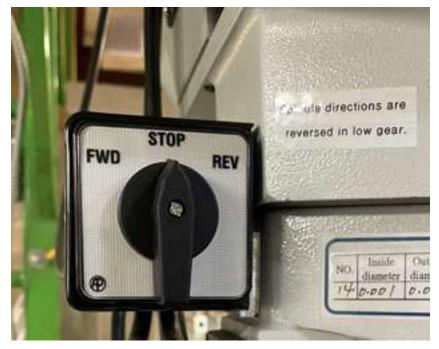
To start the mill, simply turn the power knob to run the spindle forward (FWD) or in reverse (REV).
