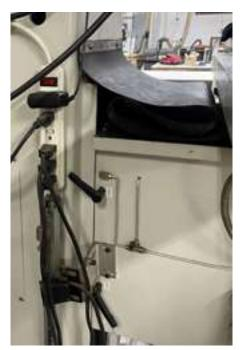
To use the mill, you'll need to power the ancillary features by turning on this power strip, attached to the mill on the left front of the main body. This will provide power to the three auto-feed motors, the DRO (location readout), a spindle light, and a coolant pump which will be installed later.
