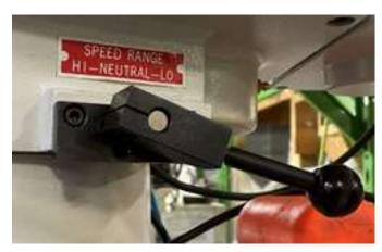
To switch to the LO gear range, push the lever inward slightly, then turn the lever back. Release the inward force and continue turning the lever back until a clear detent is reached.
