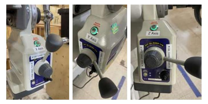
Just like the Rong Fu's feed, these have auto-stops at both ends. However, unlike the Rong Fu, these aren't the hard limit stops for the table travel. You can go a bit further using the manual handles, but this should generally be avoided. Care should thus be taken using manual feed near the table limits.
