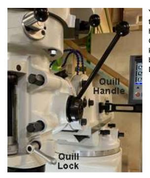
You can raise and lower the quill just like a drill press, with this handle. Like a drill press, and unlike the Rong Fu, it has a spring which will retract it whenever it isn't locked. Generally, you'll use this only for drilling. You will want to keep it locked in a single position for milling operations, because moving it invalidates the Z values shown in the DRO.
