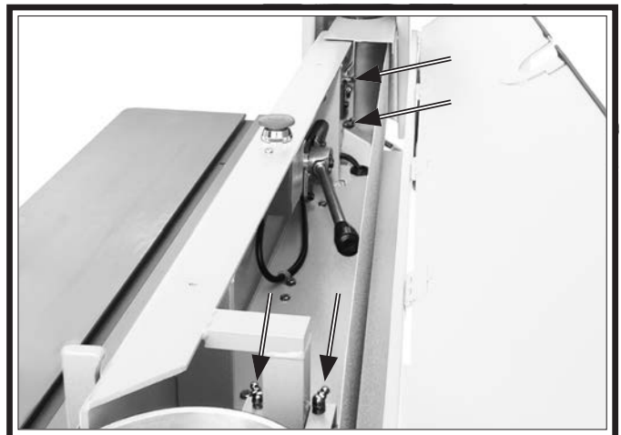
Figure 75. Location of grease fittings inside sanding body.
