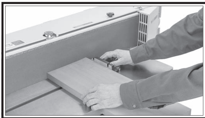
Figure 48. Typical end-sanding operation.
