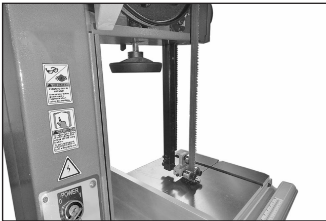
Figure 102. Guide post guard removed.
