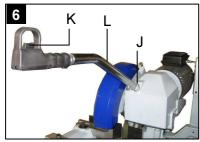
Attach the control handle to the head assembly.
