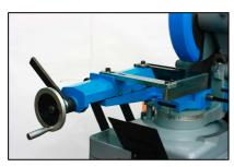
A clamping system that provides the basic support and security for the work material. Operations are conducted by hand-wheel, which opens and closes the vise jaws. The clamping vise can be adjusted forward and backward to clamp workpiece of various sizes.
