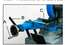
Use the hand wheel to open and close the vise jaw for work pieces that vary in width.
