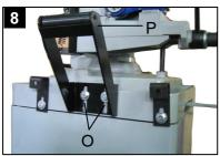
Attach the support roller to the left side of the base.
