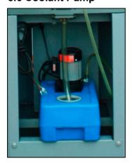
Found within the machine stand, the coolant pump is a self contained system that includes a tank, pump motor, filters and hoses.
