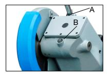
Remove the connecting plug from the electric box and unscrew the control handle.
