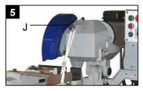
Use a wrench to unscrew a M20 X 40 hex head screw (J) from the oil fill hole (J).
