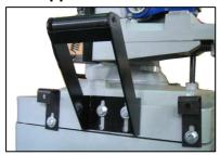
A Device that support longer sized material. The roller assists stock moving through the vise.
